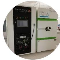
$\text{Eu}_2\text{O}_3$  thin films with thickness of 40 nm were deposited at 150  $^\circ\text{C}$  substrate temperature by using electron beam (e-Beam) evaporation.
